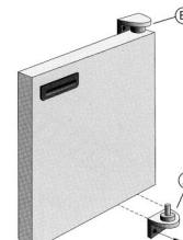
**Removal:** Unscrew the two screws holding the bottom hinge bracket **A**.
